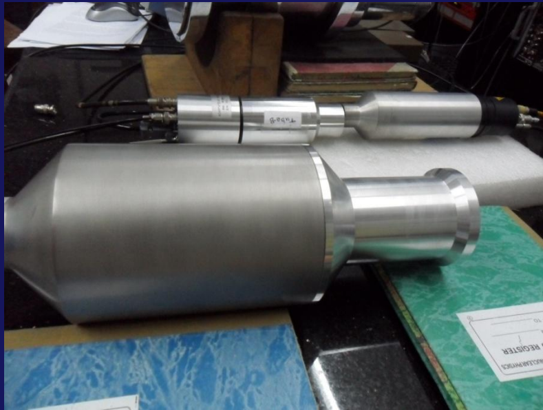
Big crystal size LaBr 3 detectors : Dimension: 7.6 cm (dia) and 15cm (length)
