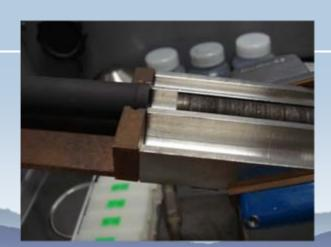
• Tests of LIST Trap: Assembled and commissioned with Ti foil target. Ga RILIS efficiency with Ti:Sa laser could not be completed. Mg beams (A=22, 23, 27), with drop in efficiency, and cleaning (>1/1e5) of Na or Al isobaric contaminants are foreseen.
