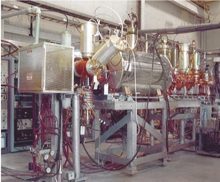
Left. BNL EBIS test stand. Suitable for HEC 2 tests and operational. Right. HEC 2 electron gun pre-assembled at CERN.
