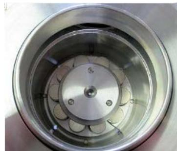
*Figure 2: Helicon source seen from the beam extraction side, with the visible first extraction stage.*
