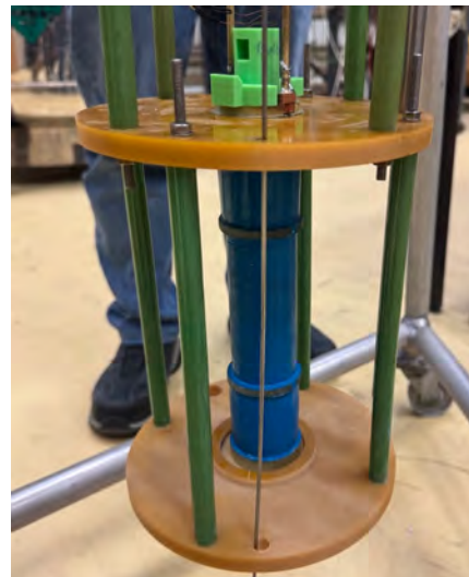
Figure 1: 2.5 T SC magnet ready for tests in CERN's Cryolab
