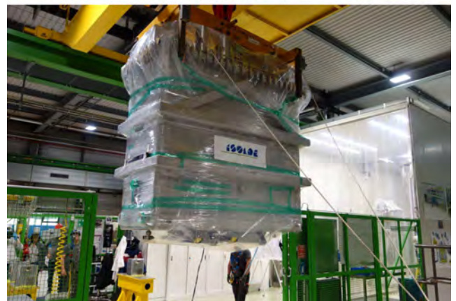
Figure 8: Top: Transport of the first HIE-ISOLDE cryomodule (CM1) from ISOLDE to the SM18 facility. Bottom: Arrival and handling of CM1 in SM18, where it will be refurbished and prepared in the clean room for future operation at ISOLDE.
