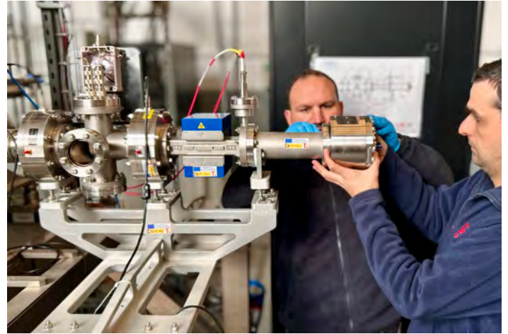
Figure 1: MHB experiment last configuration assembly process. From left to right: ACCT, MHB, ACCT, WF, FFC
