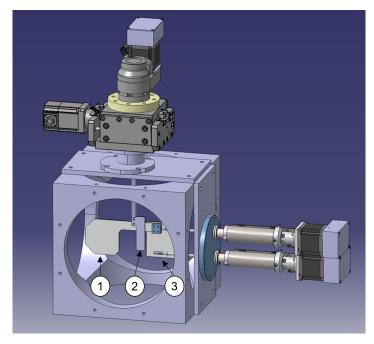
Figure 2: Schematic representation of the double collection slit system at MEDICIS. The left (1), center (2) and right (3) slits are all independently controlled by 3 different stepper motors from Nanotech<sup>®</sup>.
