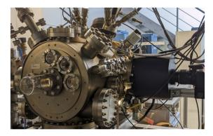
Figure 1: The ASPIC setup, being upgraded at the Georg-August-University Göttingen. The main body of the chamber has a diameter of around 330 mm (i.e., DN275), and depth of 600 mm. Source: [3].
