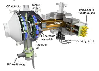
Figure 1: Reconstruction of the SPEDE detector chamber highlighting the main parts of the set-up. Reproduced with kind permission of The European Physical Journal (EPJ) [1].
