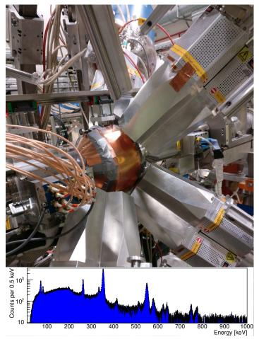
Figure 1: The Miniball array surrouding the SPEDE target chamber. The gamma-ray energy spectrum associated with Coulomb excitation of <sup>182</sup>Hg is shown at the bottom.
