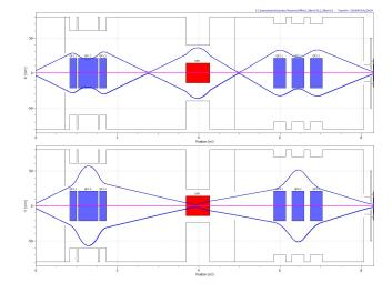
Figure 1: Beamline envelopes in the horizontal and vertical plane of the Offline 2 facility from the ion extraction electrode to the entrance of the RFQ.
