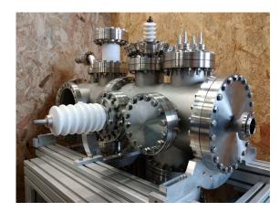
Figure 2: The ASCII chamber, now at ISOLDE-CERN, being prepared for installation. Photo taken in February 2023. Source: the authors.
