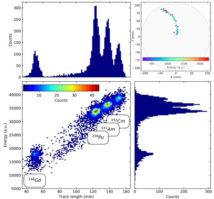
Figure 2: Spectra of  $\alpha$ -particles emitted by a quadrupole  $\alpha$  source based on the length of spiral tracks and the amount of ionisation electrons generated by the particles along the tracks (energy). An example of an  $\alpha$ -particle track recorded in a 2.5T magnetic field is shown in the top right panel.
