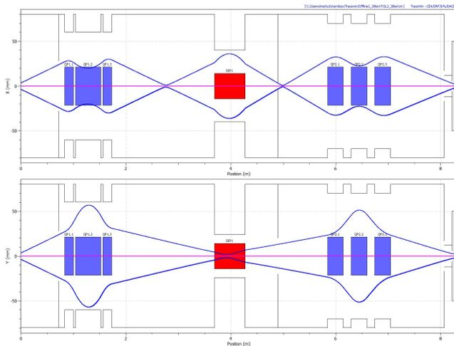
Figure 1: Beamline envelopes in the horizontal and vertical plane of the Offline 2 facility from the ion extraction electrode to the entrance of the RFQ.
