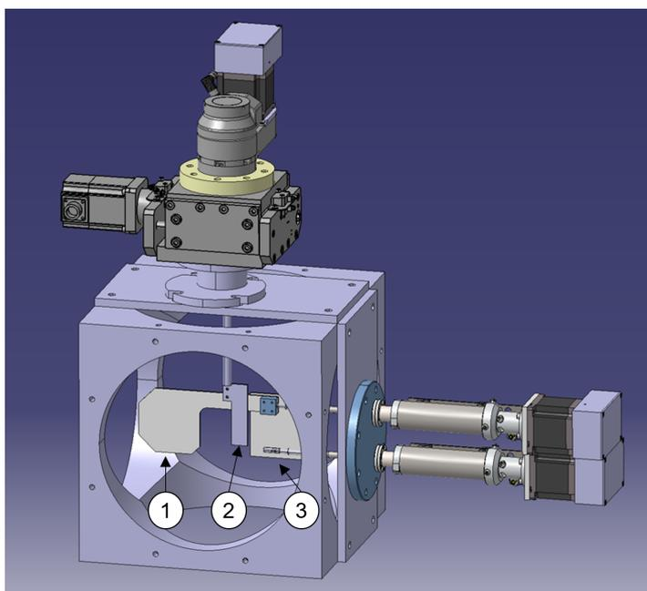
Figure 2: Schematic representation of the double collection slit system at MEDICIS. The left (1), center (2) and right (3) slits are all independently controlled by 3 different stepper motors from Nanotech®.
