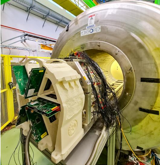
Figure 1: The SpecMAT active target at ISOLDE.
