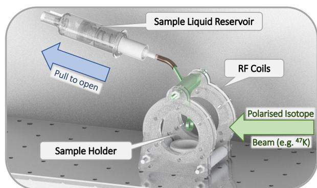
Figure 1: Rendering of the new liquid sample holding system including the sample holder and the sample liquid reservoir, openable from the outside.
