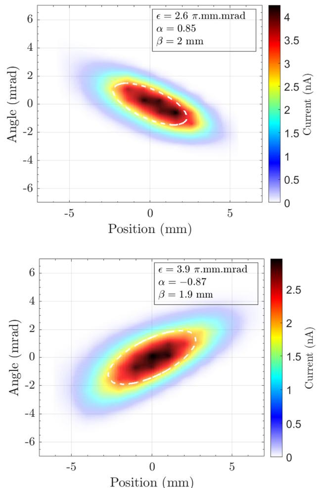
Figure 1: Transverse phase space measured from both emittance meters installed at the end of the RC6 beam-line.
