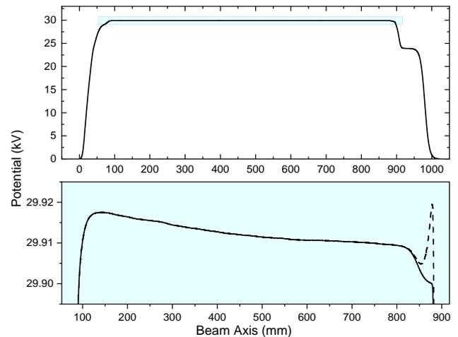
Figure 2: Longitudinal DC potential along the full RFQcb beam axis in transmission mode (solid) and bunching mode (dashed). The graph below shows a zoom on the inner ramped DC field where the RF field is present.
