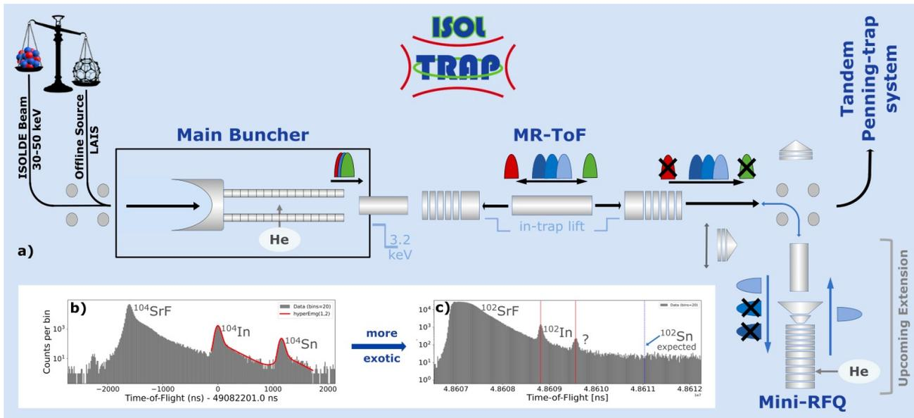
Figure 2: A schematic of the current setup of ISOLTRAP is displayed in (a) together with the upcoming extension by the Mini-RFQ. Inset (b) presents the ToF spectrum of the isobaric mass separation at  $A = 104$ , where the tails of each mass peak are clearly visible. Inset (c) displays the ToF spectrum of more exotic neutron-deficient  $^{102}\text{Sn}$ , where tails of contamination such as SrF impede the mass measurements.
