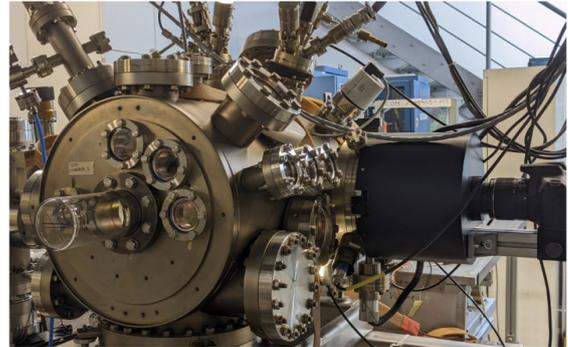
Figure 1: The ASPIC setup, being upgraded at the Georg-August-University Göttingen. The main body of the chamber has a diameter of around 330 mm (i.e., DN275), and depth of 600 mm. Source: [3].
