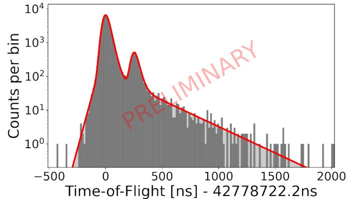
Figure 1: Time-of-flight spectrum for the  $A = 79$  ISOLDE beam from a  $\text{UC}_x$  target with quartz transfer line and laser ionization tuned for zinc. The ground (left) and isomeric (right) states are well separated.
