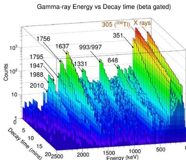
**Fig.2:** Gamma-ray transitions in prompt coincidence with beta decay. Transitions associated with  $^{207}\text{Tl}$  are distinguishable from the few contaminants by their characteristic decay time ( $t_{1/2} = 2.9$  mins).
