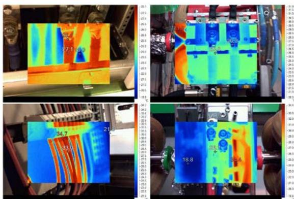
*Fig.8: IR pictures taken from the 13 hours heat run of the quadrupole and steerer magnets in XT00 line.*
