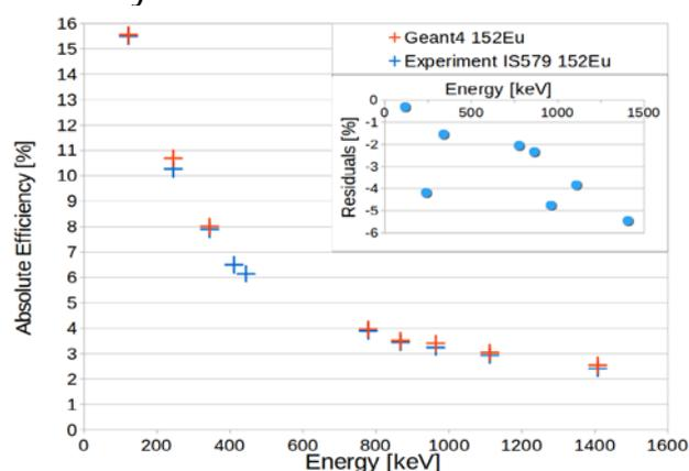
**Fig.2** Comparison between experimental and simulated photopeak efficiencies for the clover array in the IS579/IS588 experiment (no add-back algorithm applied). The inset shows the discrepancies between the data and the simulation.
