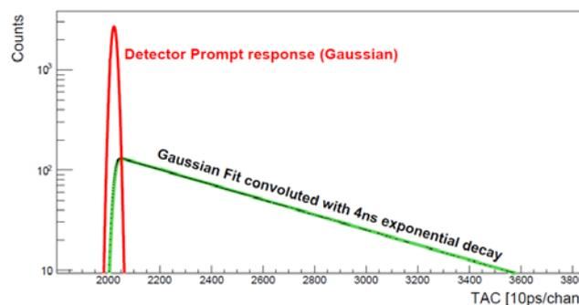
**Fig.4:** Comparison between the gaussian response of the fast-timing setup and the time distribution expected for a nuclear level of 4ns half-life.
