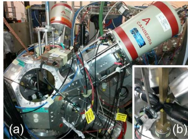
**Fig. 2:** (a) Detection system of IDS during the IS590 experiment; (b)  $\gamma$  and  $\beta$  detectors in close geometry around the implantation point.
