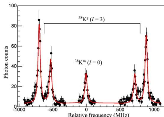
*Fig.1: Hyperfine spectra for two states in  $^{38}\text{K}$  shown relative to the centroid of the ground state. Four peaks are obtained for the ground-state with  $I = 3$ , while the single peak in the middle belongs to the isomeric state with  $I = 0$ .*
