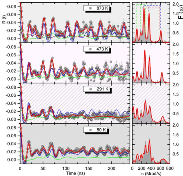
**Fig.1:** Representative  $R(t)$  functions, corresponding fits (Partial fits, corresponding to each individual EFG, are represented in blue and green and the sum in red) and respective Fourier transform taken at different temperatures using the <sup>111</sup>Cd probe.
