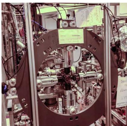
*Fig. 1: The setup of the four  $\text{LaBr}_3$  gamma detectors around the sample.*
