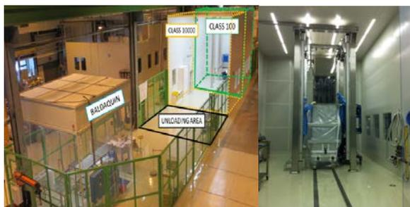
**Fig.4:** Cryomodule Assembly area equipped with specific toolings (CERN-SM18).
