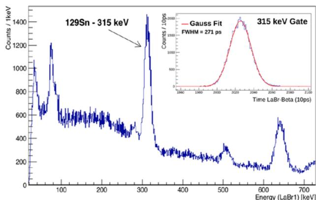
**Fig.3:** Experimental LaBr3(Ce)  $\beta$ -gated energy spectrum and (inset) time distribution of the 315-keV peak from  $^{129}\text{Sn}$ .
