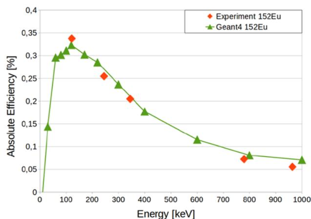
**Fig.2** Comparison between experimental and simulated photopeak efficiencies for LaBr<sub>3</sub> detector (<sup>152</sup>Eu source placed at 100 mm).
