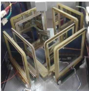
**Fig.1:** Charged particle detector setup. The beam was collected in a carbon foil located at the middle of the detector setup.
