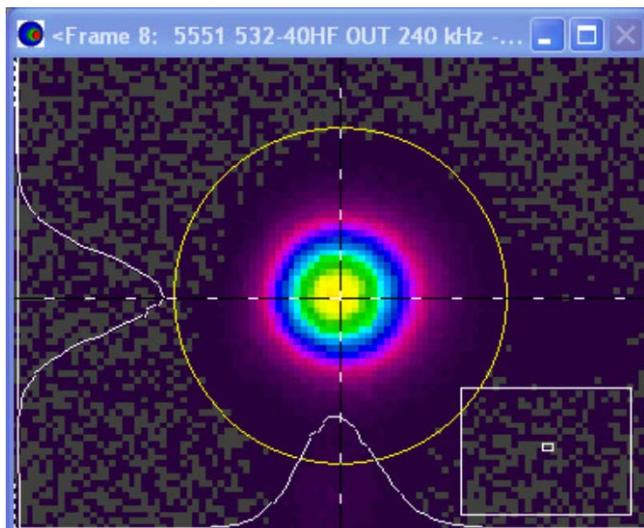
**Fig 1.** The beam profile of the Coherent Blaze laser.
