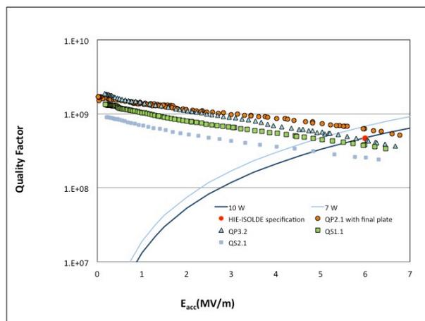
**Fig.5:** RF Test results (first four series).
