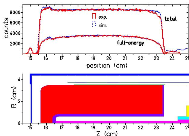
**Fig.1:** Scan with a collimated  $^{137}\text{Cs}$  source along the detector axis. Experiment and Monte-Carlo simulations are compared for the full-energy peak and the total spectrum. The lower part shows the detector model.
