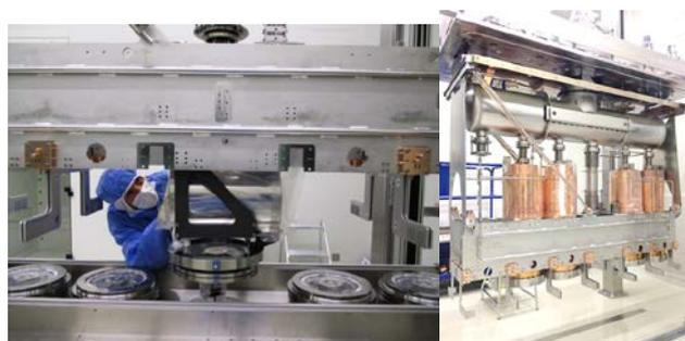
**Fig.6:** HIE-ISOLDE Superconducting Solenoid#1 being installed (left); Final assembly of the first four series cavities (right).
