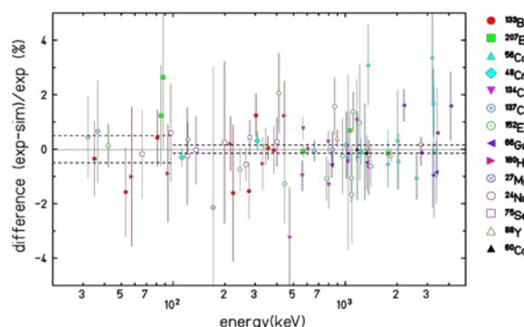
**Fig.2:** Comparison between experimental results and simulations for a large variety of sources. The lines give the adopted precision.
