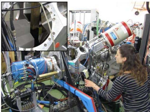
**Fig.1:** The IDS, comprised of one Miniball cluster (left) at zero degrees and four Clover Ge detectors (right). Three plastic scintillator detectors (inset) surround the implantation position.
