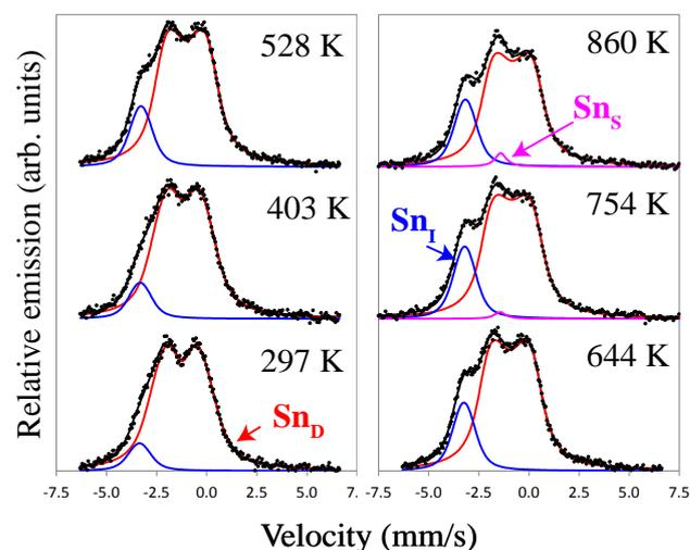
*Fig.2:  $^{119}\text{Sn}$  emission Mössbauer spectra obtained after implantation of  $^{119}\text{In}$  ( $t_{1/2} = 2.4$  min.) into CVD diamond sample held at the temperatures indicated.*
