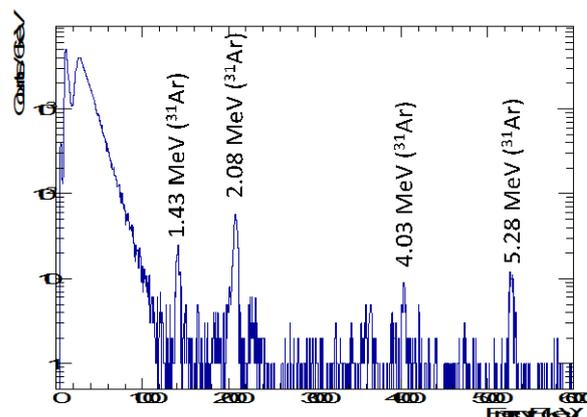
**Fig.2:**  $\beta$ -delayed proton spectrum from  $^{31}\text{Ar}$  (only small part of the data recorded is shown). Several proton lines from the decay are observed.
