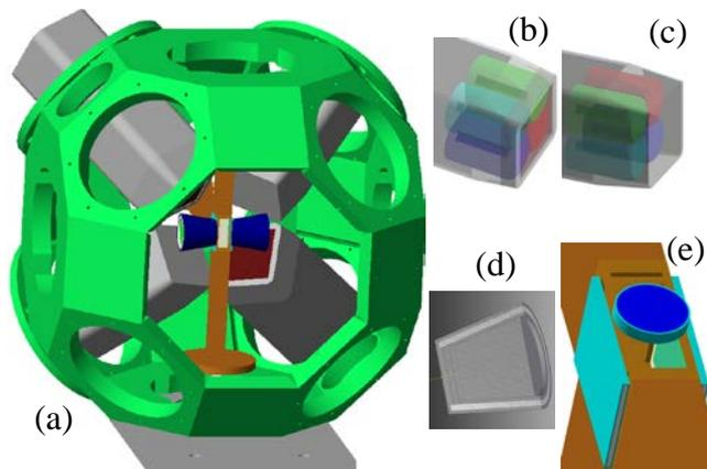
**Fig.1** (a) Representation of the fast timing configuration; (b) Ge clover detector with carbon epoxy foil; (c) and Al front cap; (d) conical LaBr<sub>3</sub> detector; (e) plastic detectors.
