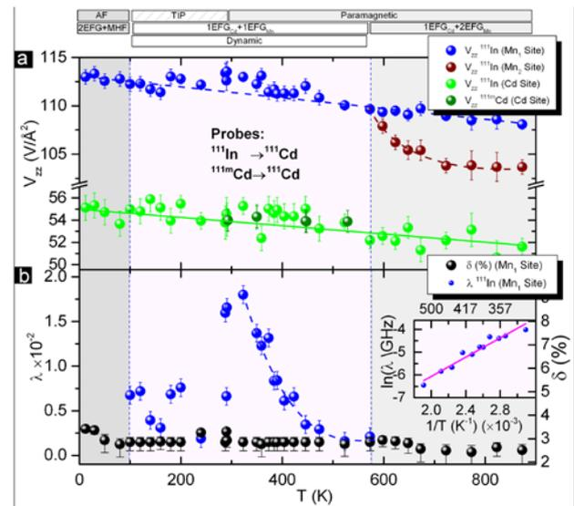
**Fig.2:** a) Experimental EFG principal component (dots). The continuous lines represent a least-squares fit of the function  $V_{zz}(T) = V_{zz}(0)[1 + aT^k]$  to the data points. b: Dynamic (left scale) and static (right scale) attenuation parameters of  $EFG_1^{Mn}$ . (inset) Natural logarithm of the dynamic attenuation parameter of  $EFG_1^{Mn}$ .
